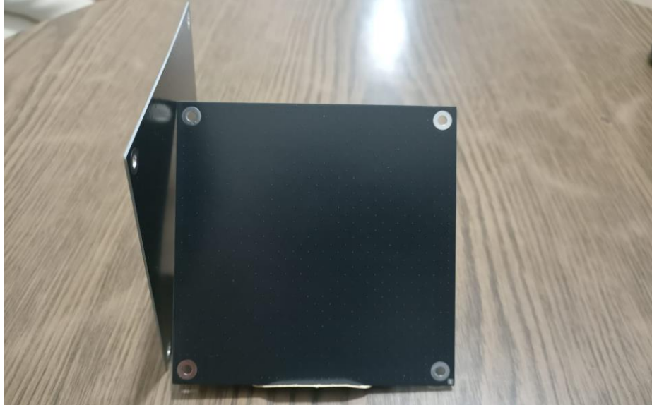
Figure 4.7: Heatsink/Damper/Spacer PCB Plates
