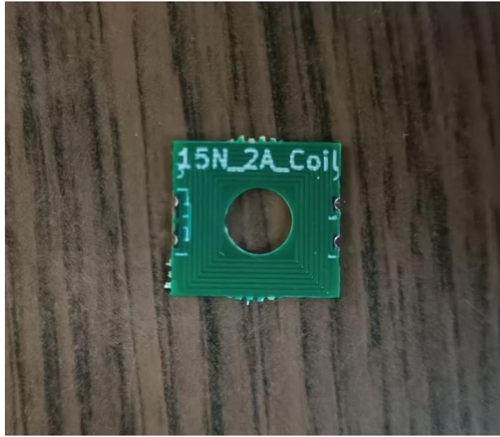
Figure 2.2: Printed planar coil.
